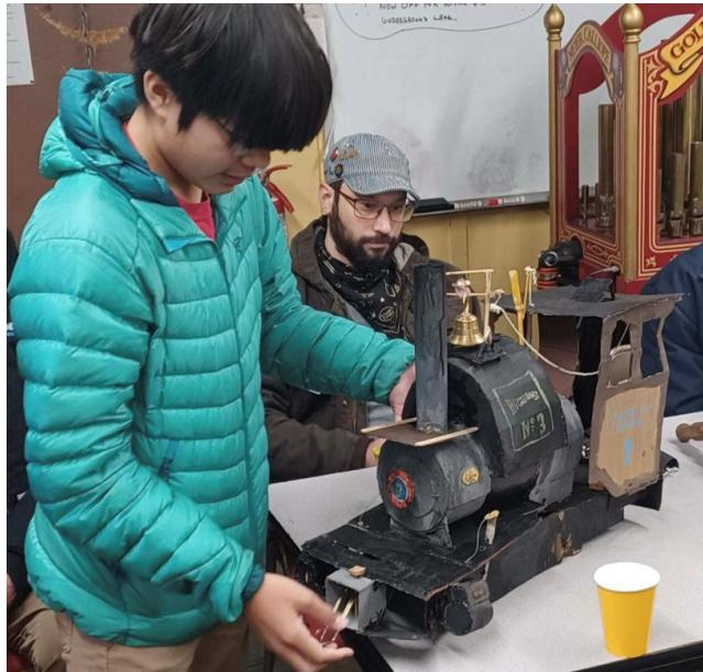
Mono Mata-Lee has been making changes to his 0-4-0 Porter saddle tank engine named Huckleberry #3. Mono felt the appearance should be weathered and using charcoal has given the engine that in-service look (a nice touch indeed). Lubrication details have been added and the wheels removed to add Hackworth valve gear, which will be completed sometime in the new year.
