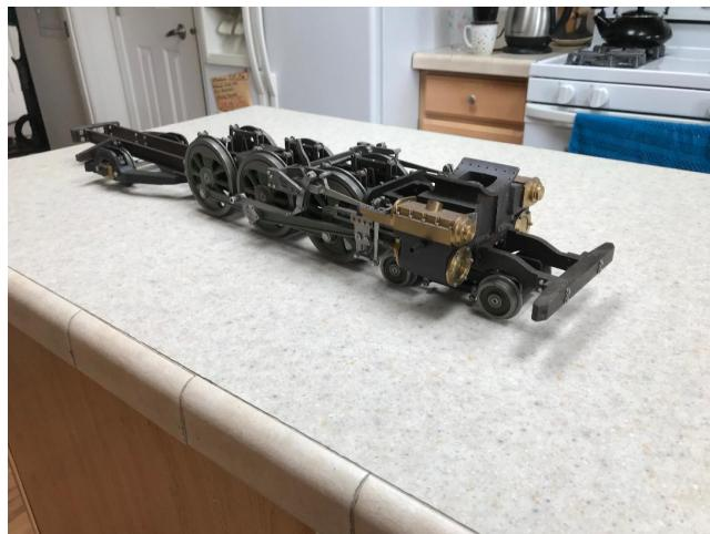
I completed the frame, wheels & all running gear plus tender frame with wheels. I had it running on air before I realized that it was the wrong scale for me and went over to Gauge 1.
