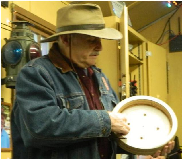
Since the tires are rubber, and therefore flexible, normal methods of work holding would not work and Charlie considered several options to hold each wheel while machining them. He finally settled on a version of what is known as a "Pot Chuck" which he made from wood, and the finished items are very nice.
