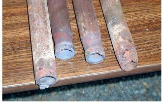
John Lisherness talked about how he removed the fire tubes and eventually cut out the club Pacific's firebox from its boiler. John then did a post-mortem analysis on how the boiler ended up in this condition and then showed the corroded components. His solution is to build a new firebox, insert rolled-in copper fire tubes and possibly reposition the firebox oil burners.
