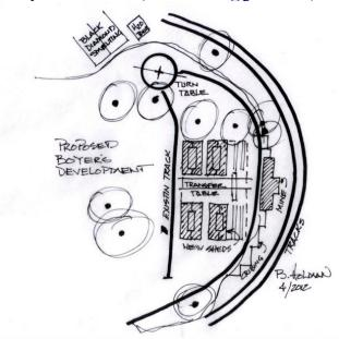
Where is that? You know, at the far end of the mainline track before you start up the elevated track out by the redwood trees. This will be another new development of the GGLS. The first phase of the project will be to reinforce the embankment with new compacted earth & cribbing and a new future roadbed.
